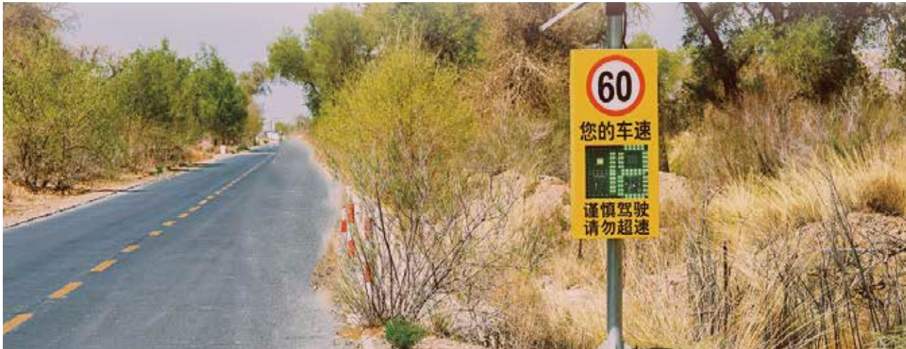
Application: Oncoming vehicle alerts, side-mounted traffic speed detection and speed feedback systems.
